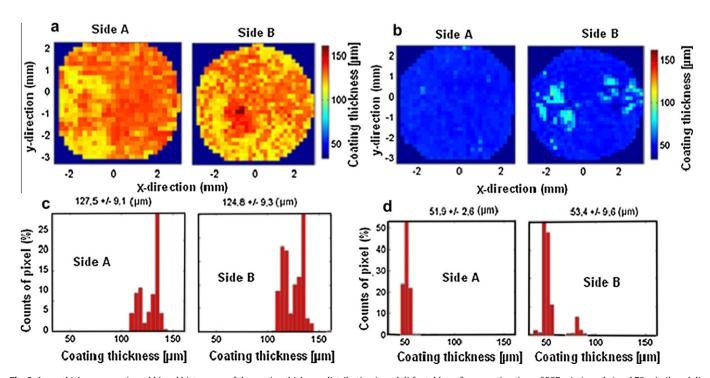
Fig. 6. Layer thickness maps (a and b) and histograms of the coating thickness distribution (c and d) for tablets after a coating time of 287 min (a and c) and 73 min (b and d).
