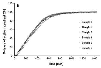
Fig. 4. Dissolution profile of samples collected after 73 min coating time (a) and at the end of the process (b).
