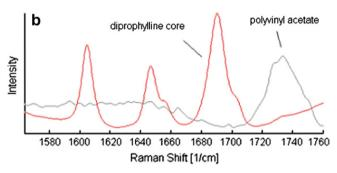
**Fig. 2.** Reproduced spectra by MCR of coating material and diprophylline core (a) compared to the Raman spectra (b). (For interpretation of the references to colour in this figure legend, the reader is referred to the web version of this article.)
