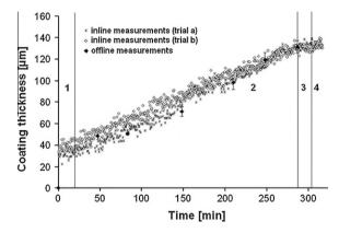
**Fig. 9.** Predicted coating thickness ( $\mu$ m) for trials A and B from in-line data (n = 10; mean ± CI 95%); process steps: 1, warm up; 2, coating; 3, drying; and 4, cooling.
