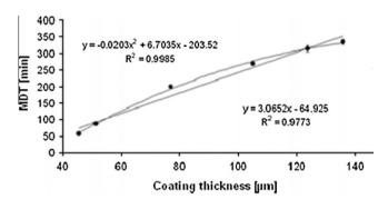
**Fig. 11.** MDT vs. coating thickness (batch A; mean; n = 6, 37–287 min).
