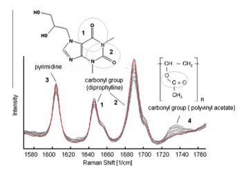
**Fig. 1.** Baseline corrected spectra of tablets during the coating process. (For interpretation of the references to colour in this figure legend, the reader is referred to the web version of this article.)
