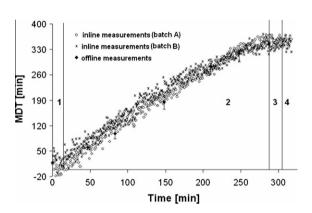
**Fig. 5.** Prediction of MDT for trials A and B from in-line data (n = 12; mean  $\pm$  Cl 95%); process steps: 1, warm up; 2, coating; 3, drying; and 4, cooling.
