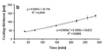
Fig. 10. MDT (a) and coating thickness (b) with coating time of batch A (n = 6; mean  $\pm$  CI 95%).
